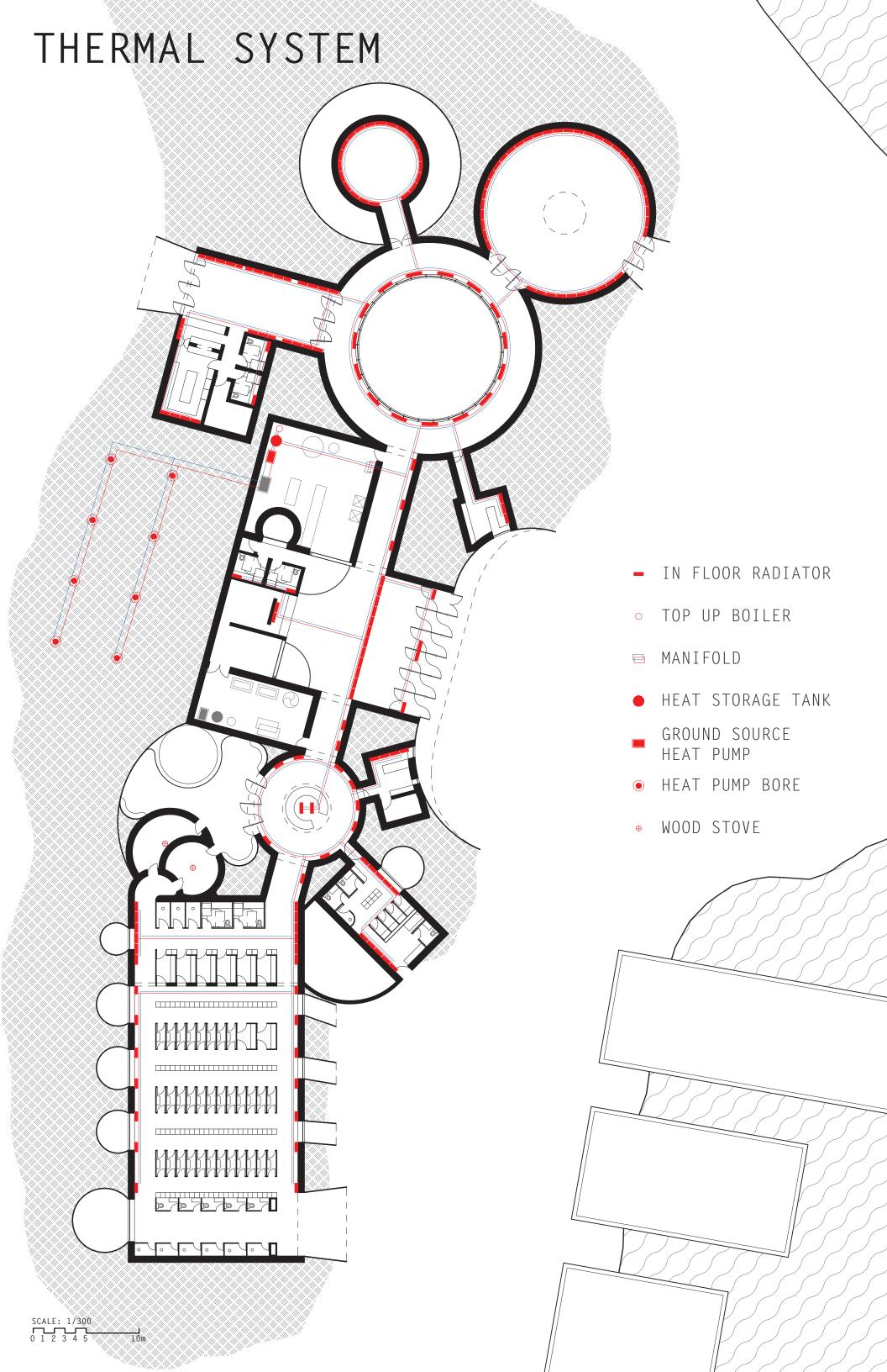
The thermal system is centralized, and takes advantage of a ground source heat pump for high efficiency. The heat pump feeds to a bore field under the shallow part of the dune, so that the bores can be dug out if needing service.
