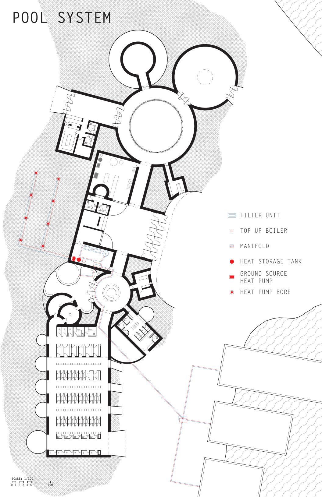
The pools also use a heat pump to acheive good effeciency. The extra step that the pools have that the thermal system doesn't is the requirement to go through a filtration and salination to treat the water. The hot tub has a seperate system after the heat pump manifold because of its diferent temperature requirement.
