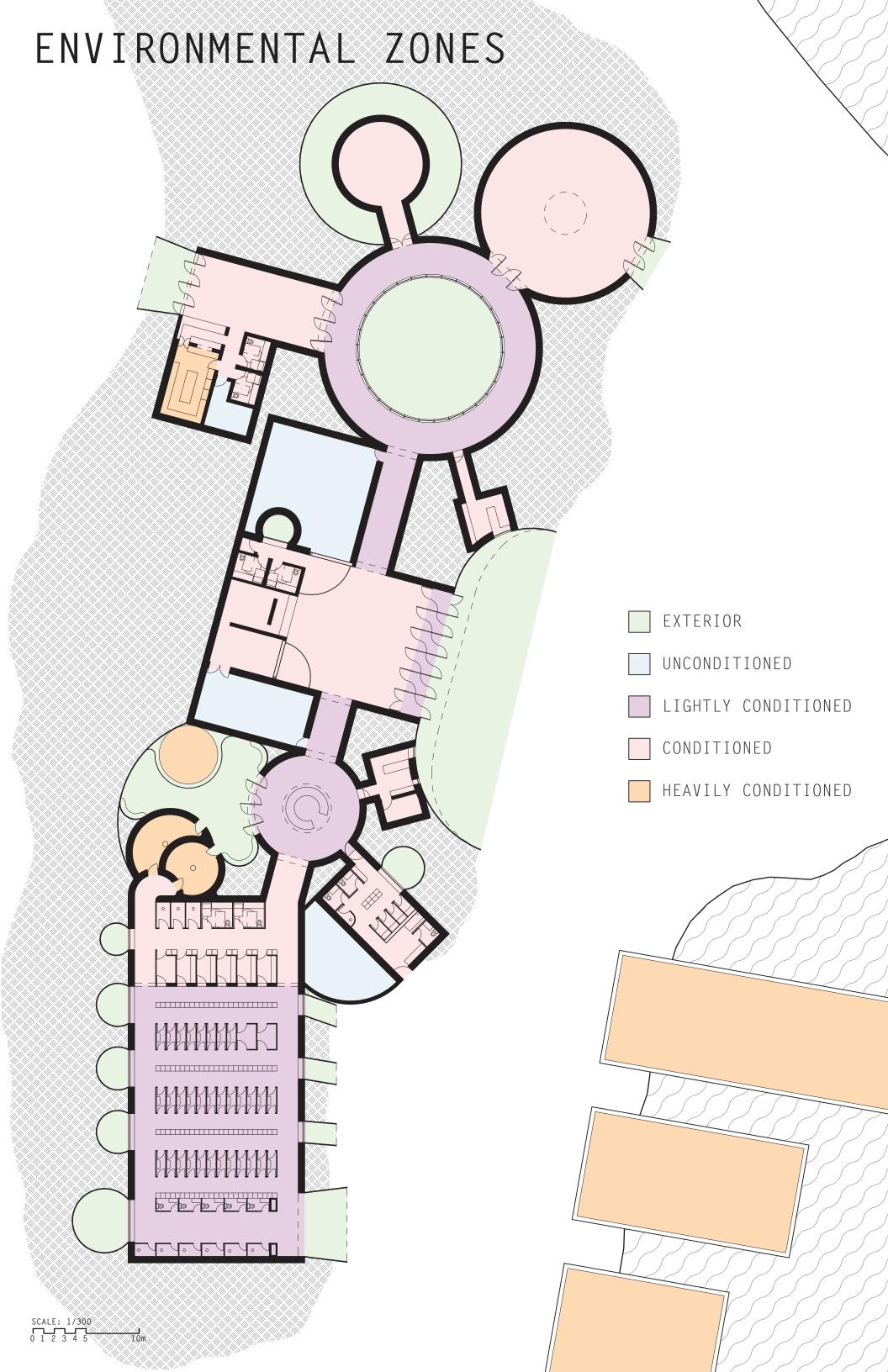
The various areas and programs of the building are depicted with their required levels of climate control. Some areas of the program, like the pools, saunas and hot tub, require extensive amounts of energy to keep them at optimal condition. On the other side, there are parts of the program that require basically no conditioning, such as storage rooms.
