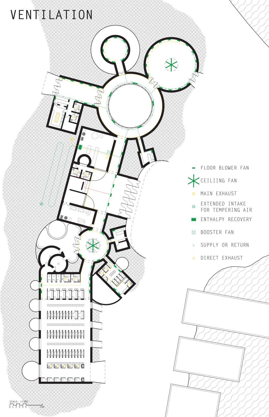
The ventilation of the building is extremely important, as this building is well sealed and the air will become stale if it isn't circulated.
