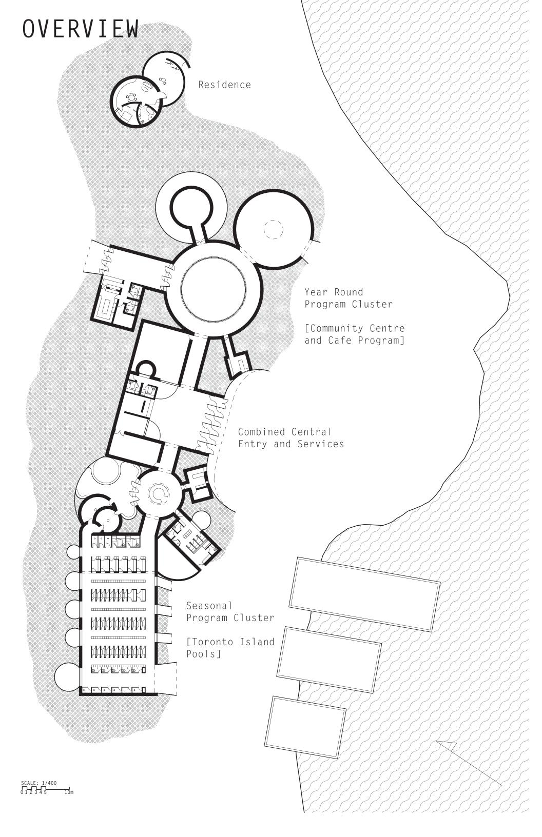
The new building still sits inside of the sand dune, and receives the same benefit of the additional insulation. The North side is very enclosed, while the South side opens up to take advantage of the Winter sun. This means that the building can have slightly less requirement for the high embodied spray foam that is used to insulate it.
